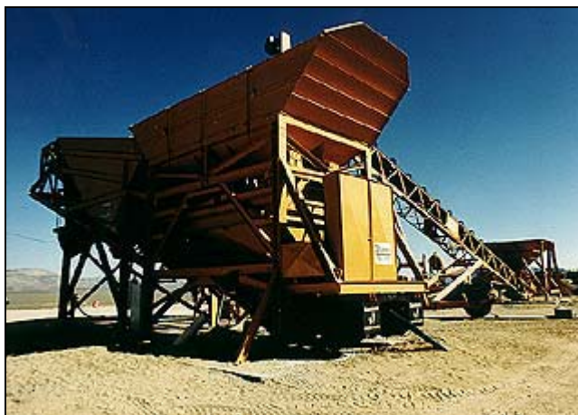
Mustang Concrete Batch Plant
