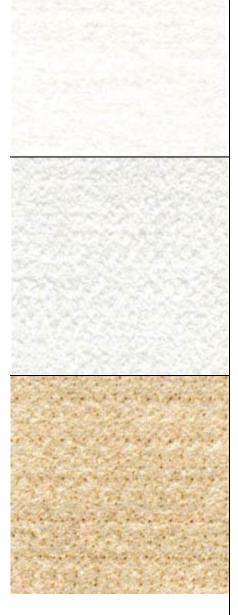
P84® Felt Polyimide Recommended continuous operation temperature: 475°F Maximum (short time) operation temperature: 500°F Supports combustion: No Biological resistance (bacteria, mildew): No Effect Resistance to alkalis: Fair Resistance to alkalis: Fair Resistance to mineral acids: Good+ Resistance to organic acids: Good+ Resistance to organic acids: Good+ Resistance to organic solvents: Excellent Available weights: 14 oz. - 18 oz.
